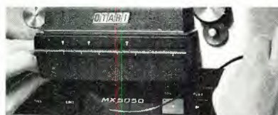
Easy threading; capstan on back side.
